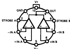
NOTE: Pin 5 connected to case.
